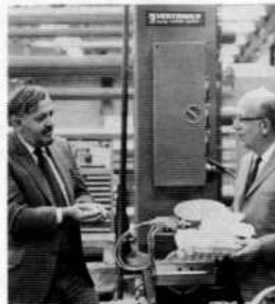
The Vertruder 4500, made by Gloucester Engineering Company, can reclaim 650 pounds of plastic scrap per hour. An upcoming version can recycle 1300 pounds per hour. Displaying the "raw material" and the finished product are Ingvar E. Tornberg, vice president, and G. Wilbur Tracey, president of Gloucester Engineering.
